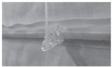
2. One inner cord breakaway clip will be used on each cord where it crosses a tape. See fig. 1.
