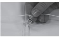
If the clip breaks apart, push the small c-clip section (which will remain on the cord) onto the front of the post part (which will remain on the tape). See fig. 2.
